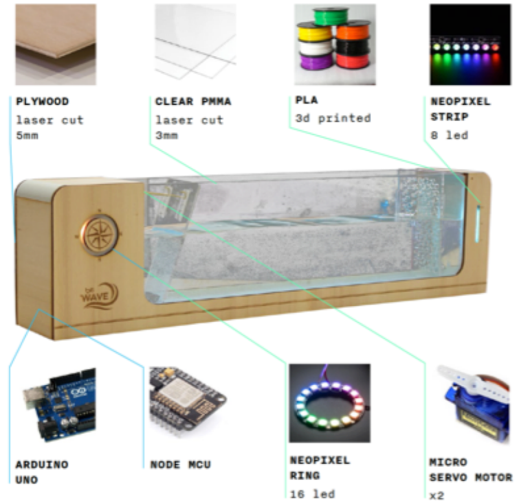
System to display tangible data about surfing: Prototyping the product using 3D printing and Arduino board and sensors
