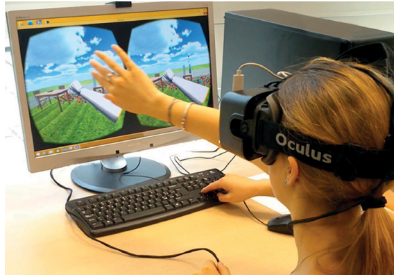
Interaction with a Virtual environment using an immersive visualization system (Oculus Rift) and Leap motion sensor
